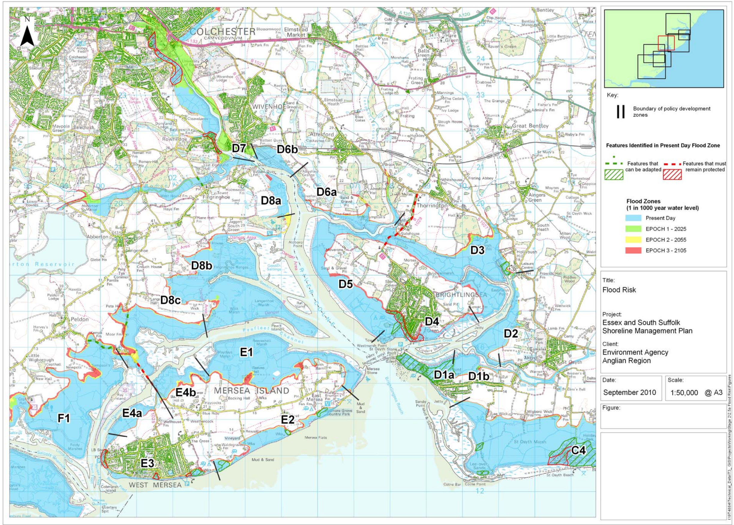
Figure 5-4 Flood Risk - Colne estuary and Mersea Island
